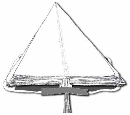
6.1.2 Fold the skirt up 90° on each side parallel to the radial seams.
